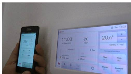
Figure 7. The display of TOON next to the application for a smartphone, products of ENECO energy company, NL
