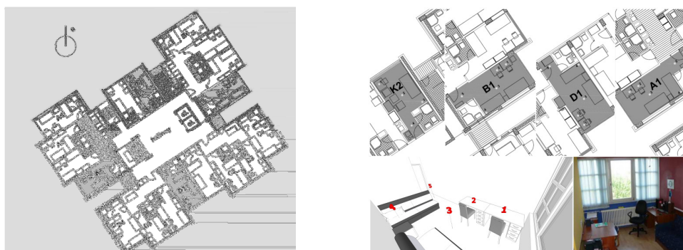
Fig 1 Student dormitory layout plan, rooms with the measurement points and appearance of one of the rooms
