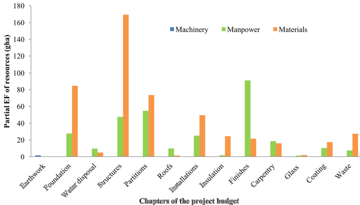
Figure 3. EF of the resources used in the construction of c49 project, residential building with 4 floors above ground and one basement floor and foundation with isolated footings.
