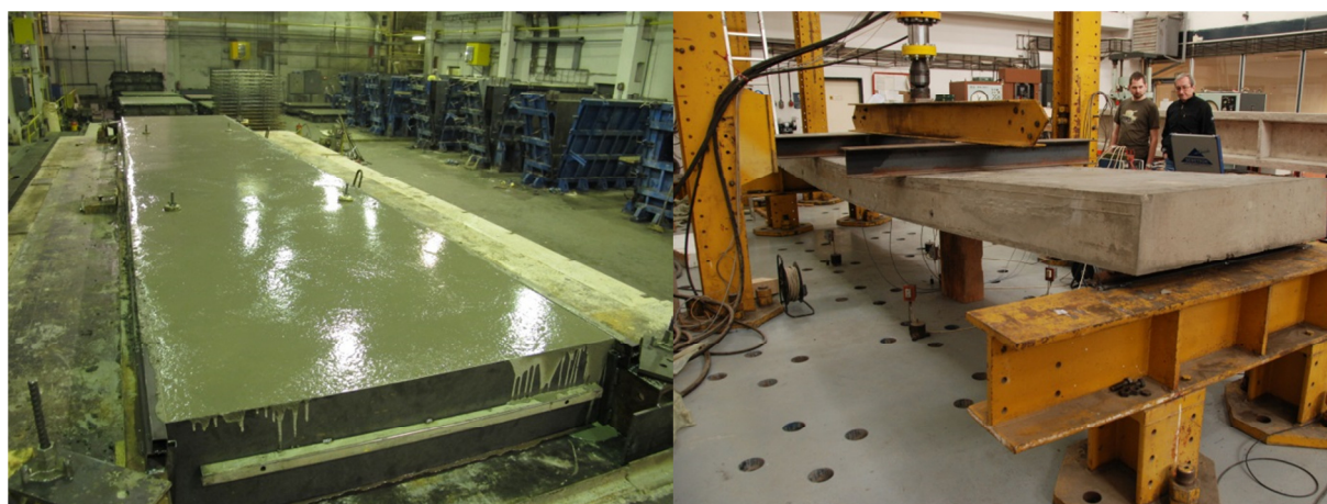
Fig. 3 Manufacturing and testing of first prototype of floor panel from HPC with lightening shell elements
